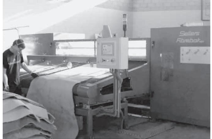
Carpet shearing machine used in recycling process.
