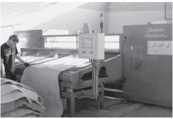
Carpet shearing machine used in recycling process.
